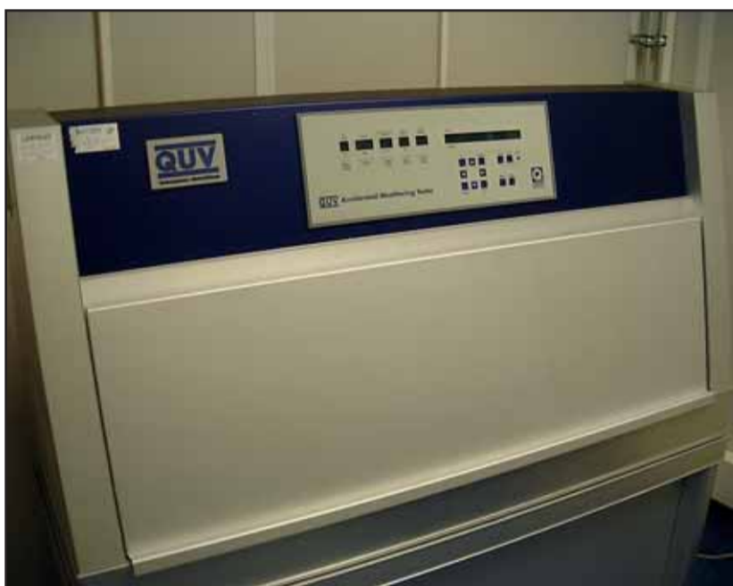
Laboratory testing equipment used to simulate weathering exposure
